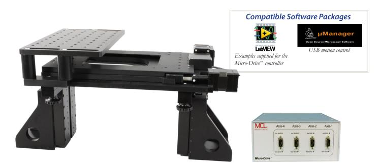
Mad-Deck<sup>™</sup> with optional breadboards for mounting probes or other accessories. Breadboard position is easily adjusted and breadboards can be removed if not needed. The Micro-Drive<sup>™</sup>4 cwith USB digital interface allows the Mad-Deck<sup>™</sup> to be conttrolled via LabView software as well as other 3rd party software.
